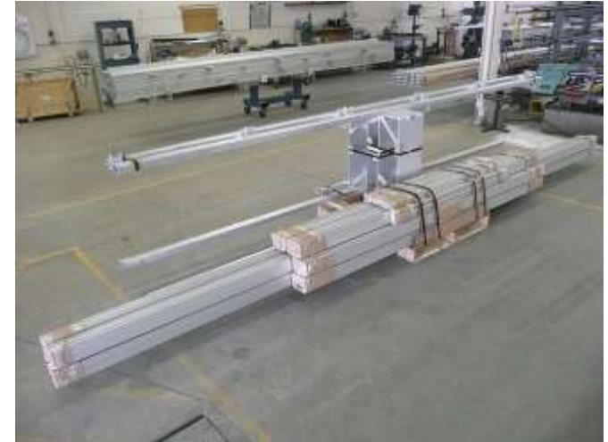
4 x PS2400F Shipping Package 4' x 4' x 20ft ~ 3050lbs 1.2 x 1.2 x 6 m ~ 1380kg
